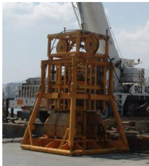
Figure 9: Example of a block push seabed CPT system (Fugro Seacalf)
