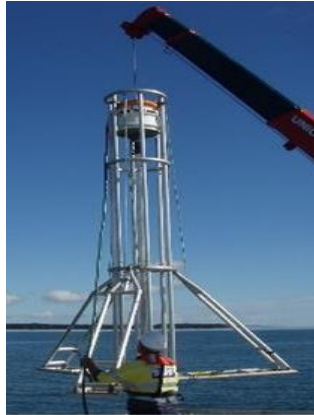
Figure 10: Example of a crane-deployed vibracore system
