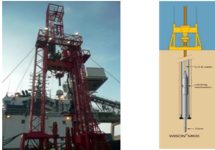
Figure 8: Borehole rig and schematic of system working.
